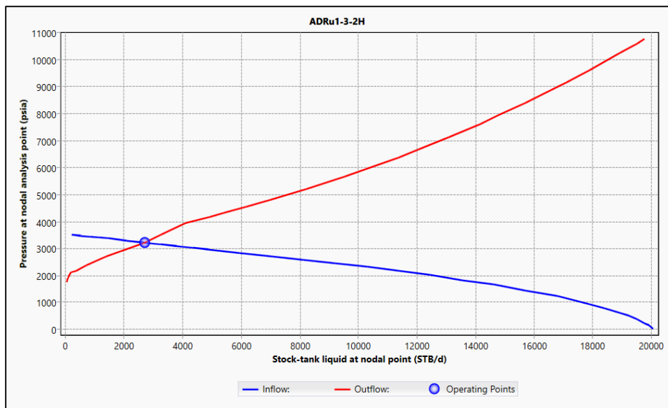
Fig. (8): The flow for well-1 after installing the gas lift system
